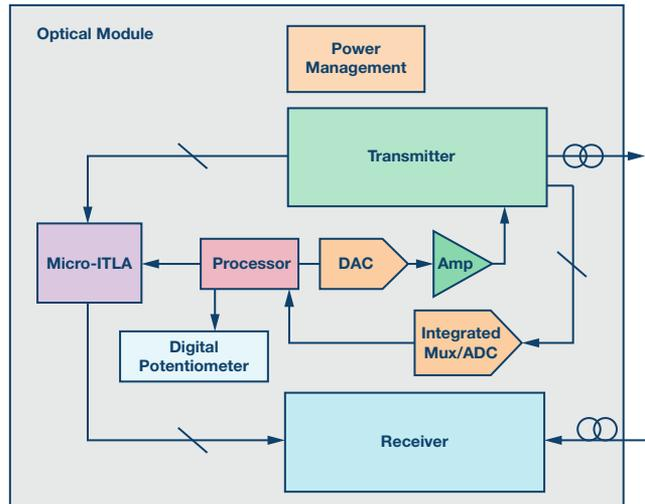
Figure 4. Simplified block diagram of an optical module.
