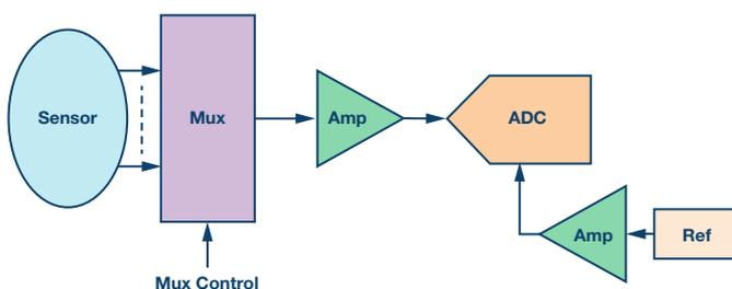
Figure 1. Simplified multichannel data acquisition signal chain case I.
