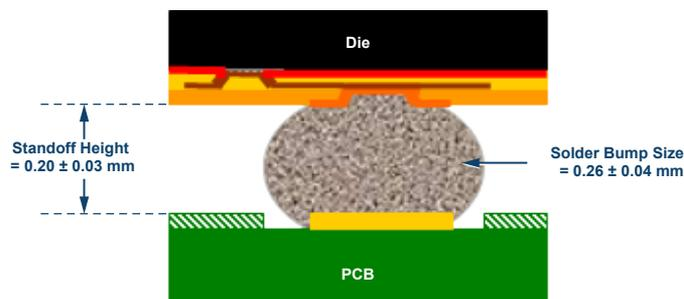
Figure 9. AD7682/AD7689 WLCS dimensions after PCB assembly.
