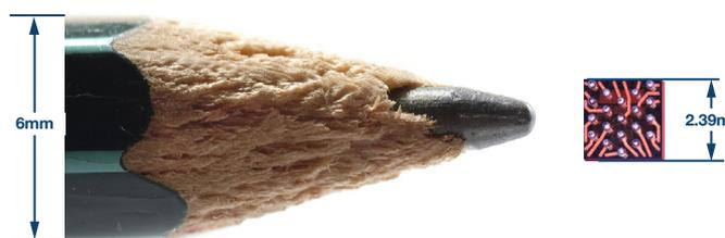
Figure 8. Size comparison of AD7682/AD7689 wafer level, chip scale package with a standard pencil.
