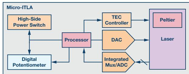
Figure 5. Simplified block diagram of a microintegrated tunable laser assembly.
