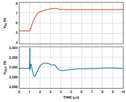
Figure 9. ADM7150 line transient response. 5 V to 7 V line step in 1.5  $\mu s$  (red). Output voltage (blue).
