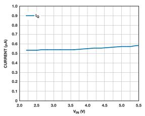
Figure 3. Quiescent current vs. input voltage of the ADP160 LDO.
