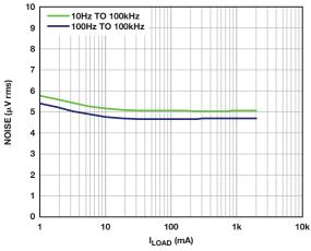
Figure 14. ADM7172 output noise vs. load current.
