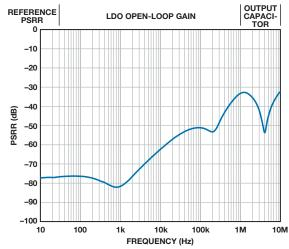
Figure 11. Typical LDO PSRR vs. frequency.
