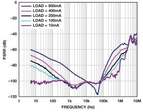
Figure 12. ADM7150 power supply rejection vs. frequency.  $V_{\rm OUT}=5$  V,  $V_{\rm IN}=6.2$  V.
