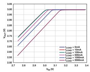
Figure 2. Dropout region of the 3.0-V ADM7172 LDO.
