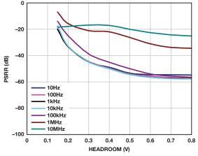
Figure 13. ADM7172 power supply rejection vs. headroom,  $V_{out} = 5$  V, 2 A load current.
