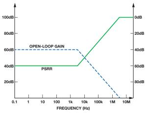
Figure 10. Simplified LDO gain vs. PSRR
