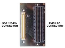
Figure 3. SDP-I-FMC interposer.
