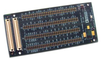
Figure 7. SDP breakout board.
