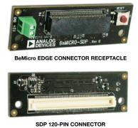
Figure 5. BeMicro SDK/SDP interposer.
