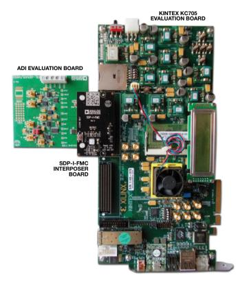
Figure 4. SDP-I-FMC interposer connects daughter board to Kintex KC705 evaluation board.
