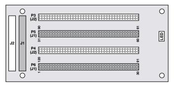
Figure 8. Top view of SDP breakout board.
