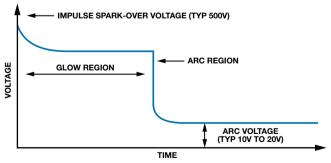
Figure 9. GDT characteristic waveform.
