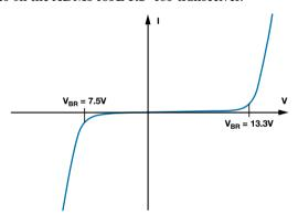
Figure 7. CDSOT23-SM712 I/V characteristic.
