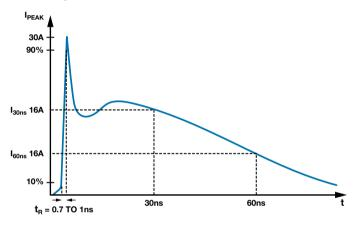
Figure 1. IEC 61000-4-2 ESD waveform (8 kV).
