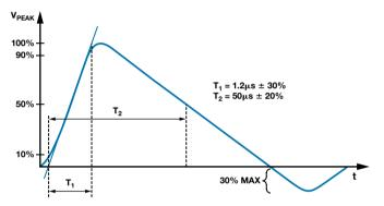
Figure 3. IEC 61000-4-5 surge  $1.2/50 \mu s$  waveform.
