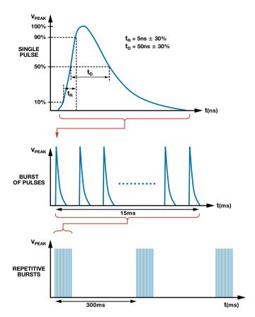
Figure 2. IEC 61000-4-4 EFT 50  $\Omega$  load waveforms.
