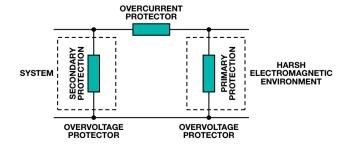
Figure 5. Protection scheme—block diagram.
