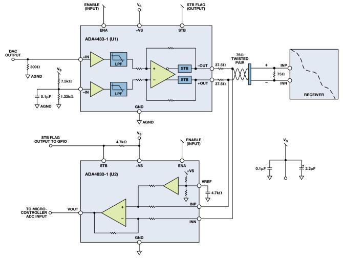
Figure 1. Wire diagnostic circuit using the ADA4433-1 (U1) and ADA4830-1 (U2).
