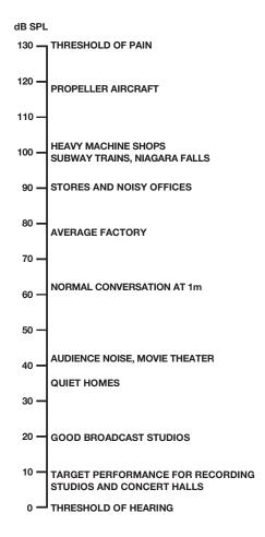
Figure 4. Sound pressure level of various sources.<sup>1</sup>
