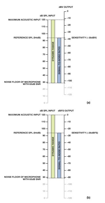
Figure 2. Mapping acoustic input level to (a) voltage output level for an analog microphone; (b) digital output level for a digital microphone.
