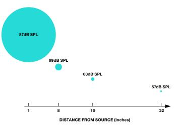
Figure 3. Sound pressure level at the microphone is reduced as the distance from the source increases.
