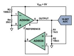
Figure 3. Higher resolution temperature measurement with offset adjustment.
