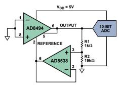
Figure 2. High-resolution temperature measurement.
