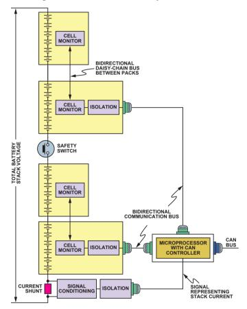
Figure 1. Serial cell monitoring and isolation in a battery stack.
