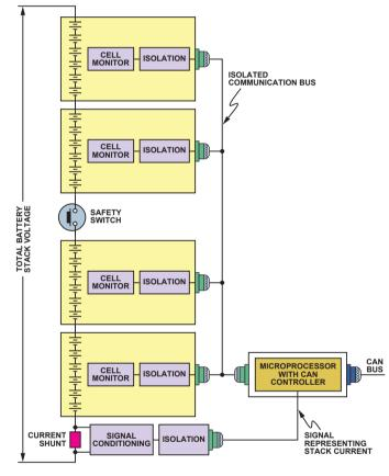
Figure 2. Battery stack with parallel access to packs.
