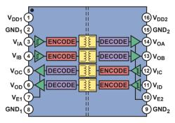
Figure 3. Functional block diagram of ADuM1402 quad isolator.
