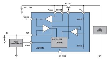
Figure 1. Running braking lamps controller.
