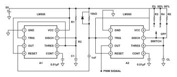
Figure 2. PWM signal generator.
