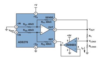
Figure 3. Simplified circuit for low-current applications.
