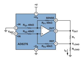
Figure 4. Simplified circuit for low-cost, low-current applications.
