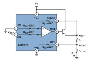
Figure 2. Simplified circuit eliminates feedback amplifier.
