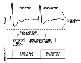
Figure 2. SINGLE\_TAP and DOUBLE\_TAP interrupts.
