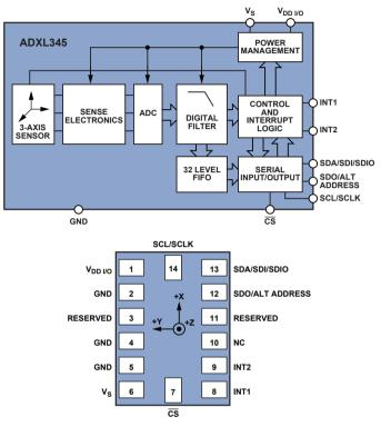
Figure 1. ADXL345 system block diagram and pin designations.
