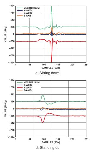
Figure 3. Accelerometer responses to different types of motion.
