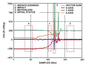
Figure 4. Acceleration change curves during the process of falling.
