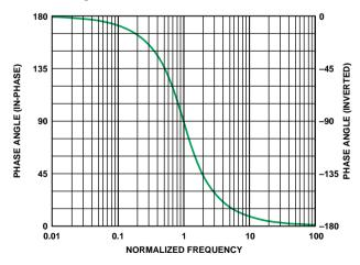
Figure 5. Phase response of a 2-pole, high-pass filter with a center frequency of 1 (in-phase response, left axis; inverted response, right axis).
