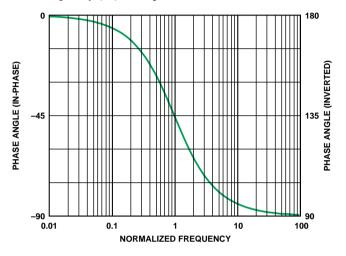
Figure 2. Phase response of a single-pole, low-pass filter about the center frequency (in-phase response, left axis; inverted response, right axis).
