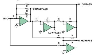
Figure 16. 2-pole biquad filter (with a high-pass section).
