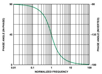
Figure 3. Phase response of a single-pole, high-pass filter with a center frequency of 1 (in-phase response, left axis; inverted response, right axis).
