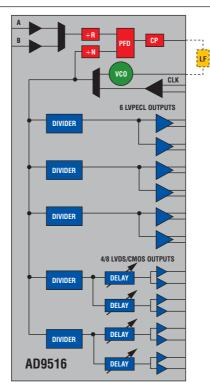
Integrated timing functions in a single 9 mm  $\times$  9 mm, 64-lead LFCSP control jitter to below 1 ps rms
