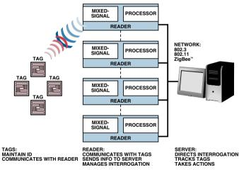
Figure 1. Simplified representation of an RFID system.
