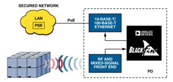
Figure 4. Example of a PoE-based RFID asset-tracking system.
