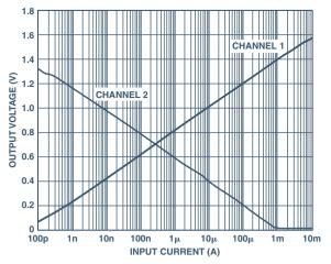
Figure 4. Transfer functions for the two outputs.
