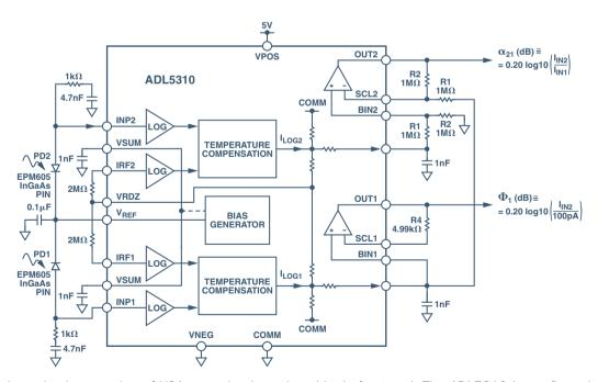
Figure 2. Hardware implementation of VOA control using a logarithmic front end. The ADL5310 is configured to provide an absolute power measurement of the optical signal power incident on PD1, while the difference voltage reveals the absorbance across the VOA. The wide dynamic range allows the loop to remain locked over a broad range of input signals.
