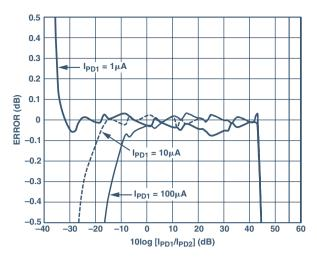
Figure 8. Log conformance for Wilson-mirror ADL5310 combination, normalized to 10- $\mu$ A Channel 1 input current,  $I_{IN1}$ .
