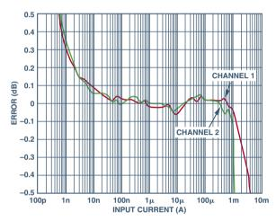
Figure 5. Log-conformance of the transfer functions.
