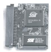
Figure 3. Inside printed circuit board of a CompactFlash (courtesy of Silicon Storage Technology, Inc.).
