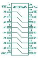
Figure 12. Flow-through pin arrangement.
