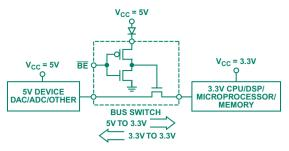
Figure 6. Using the ADG3257 to switch and level translate between a 3.3-V controller and 5-V data converter.
