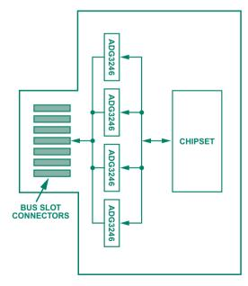
Figure 10. Hot swapping with the ADG3246 bus switch.
