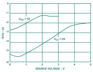
Figure 9. Charge injection for a typical bus switch (ADG3257).
