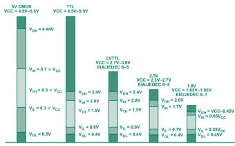
Figure 8. Logic levels compared for different supply voltages.
