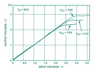
Figure 7.  $V_{\text{OUT}}$  vs.  $V_{\text{IN}}$  for the ADG3257 bus switch with  $V_{\text{CC}}$  in the 3-V range.
