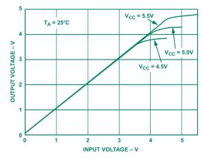
Figure 3.  $V_{\text{OUT}}$  vs.  $V_{\text{IN}}$  for the ADG3257 bus switch with  $V_{\text{CC}}$  in the 5-V range.
