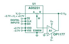
Figure 1. Programmable amplifier/attenuator.
