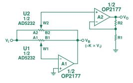
Figure 2. Bipolar programmable-gain amplifier with linear step adjustment
