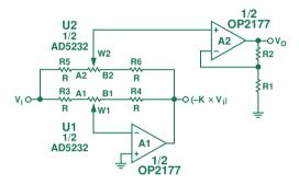
Figure 3. PGA handles high input voltage.
