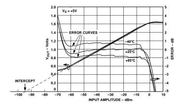
The figure also shows plots of deviations from the ideal, i.e.,  $\log conformance$ , at  $-40^{\circ}$ C,  $+25^{\circ}$ C, and  $+85^{\circ}$ C. For example, at  $+25^{\circ}$ C, the log conformance is to within at least  $\pm 1$  dB for an input in the range -2 dBm to -67 dBm (over a smaller range, the log conformance is even better). For this reason, we call the AD8313 a 65-dB log amp. We could just as easily say that the AD8313 has a dynamic range of 73 dB for log conformance within 3 dB.
