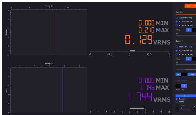
Figure 4. rms voltage across the loudspeaker.
