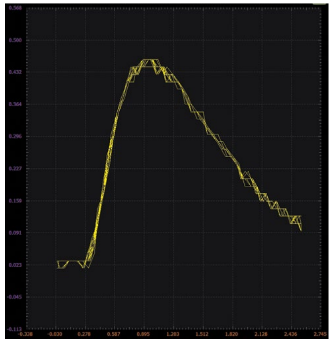
Figure 4. Q2 collector current vs. W1 voltage Scopy plot.
