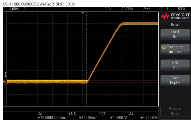
Figure 4. The LT8640. C8 = 0.1μF, with a startup time of ~50 ms for 0 A (yellow) and 4 A (brown) load currents.
