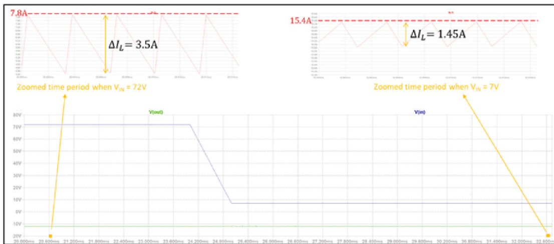
Figure 10. Measuring \Delta I_L at V_{IN} = 7\text{ V} and 72\text{ V} and extracting the peak coil current with the previous LTspice circuit.
