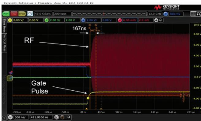
Figure 4. Measured HPA turn-on time.
