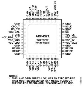
Figure 6. Pin Configuration
