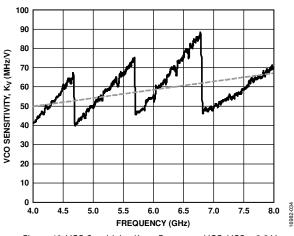
Figure 40. VCO Sensitivity, K<sub>V</sub> vs. Frequency VCC\_VCO = 3.3 V
