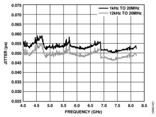
Figure 27. RMS Jitter, Fractional-N, f<sub>PFD</sub> = 153.6 MHz, VCC\_VCO = 5 V
