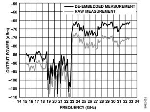
Figure 31. RF 32P and RF32N Output Power When Disabled, De-Embedded Board and Cable Measurement, Combined Using Balun
