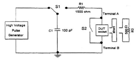
Figure 1 — Typical equivalent HBM ESD circuit
