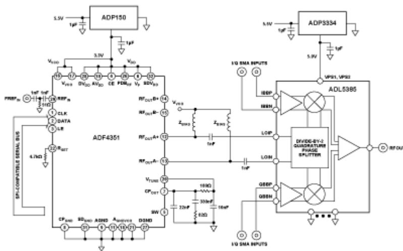
**Figure 1. Direct Conversion Transmitter (Simplified Schematic: All Connections and Decoupling Not Shown)**
