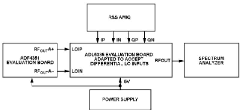
**Figure 3. Sideband Suppression Measurement Test Setup (Simplified Diagram)**
