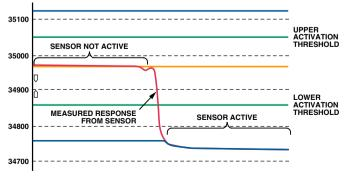
Figure 8. Typical response from a button sensor.
