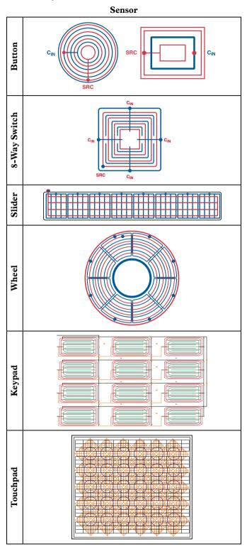
Figure 7. Selection of capacitance sensors.
