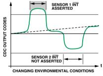
Figure 5. Sensor activation with changing ambient capacitance.
