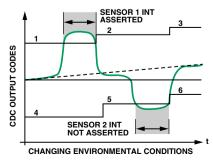
Figure 6. Sensor activation with auto-adapting thresholds.
