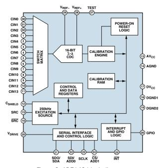
Figure 3. AD7142 block diagram.
