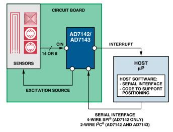
Figure 2. Three-part capacitance-sensing solution.
