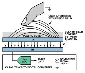
Figure 1. Sensing capacitance.
