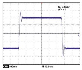
Figure 12. AD8698 output response without compensation.
