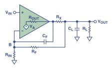
Figure 3. In-the-loop compensation circuit.
