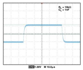
Figure 7. AD8510 output response with compensation.
