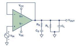
Figure 11. The  $R_S$ - $C_S$  load forms a snubber circuit to reduce the phase shift caused by  $C_I$ .
