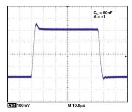
Figure 13. AD8698 output response with snubber network.
