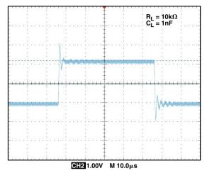
Figure 6. AD8510 output response without compensation.
