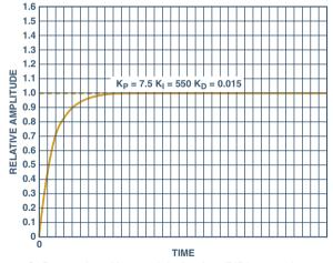
Figure 8. Proportional-integral-derivative (PID) control response.
