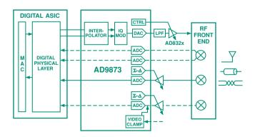
Figure 6. Broadband modems over cable, power line, or wireless, using the AD9873.
