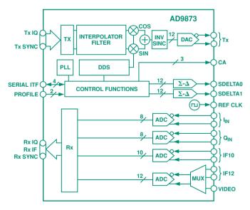
Figure 3. AD9873 functional block diagram.
