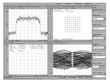
Figure 9. AD9873 64-QAM constellation plot.
