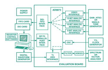
Figure 10. AD9873 evaluation setup.
