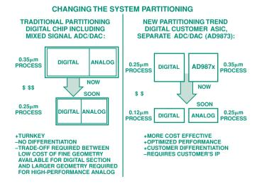
Figure 5. Smart partitioning model.
